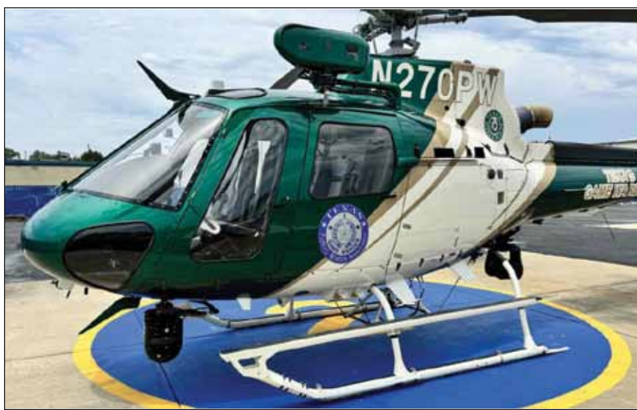
The aircraft is outfitted with the latest law enforcement technology and emergency response equipment, including a rescue hoist, thermal imager, searchlight, public address system, satellite communication, night vision and firefighting equipment.
